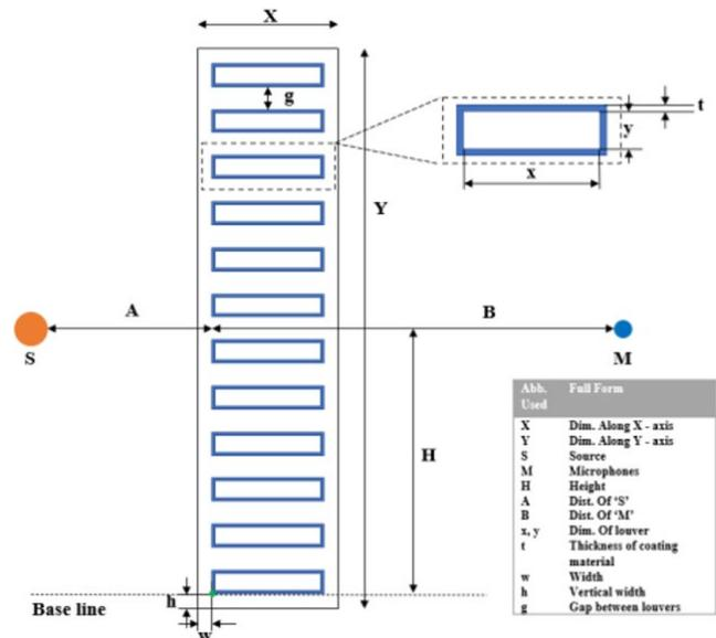
Figure 1: Schematic of louver arrangement
