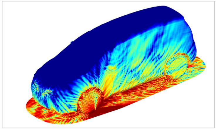
Acoustic Radiation of Tire Noise at 5000Hz
