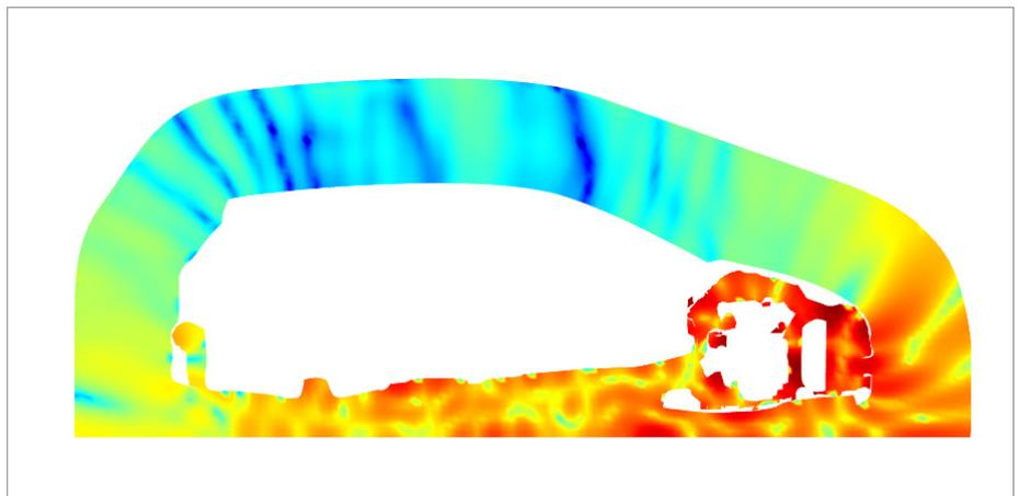
Engine Acoustic Radiation (Cut View)
