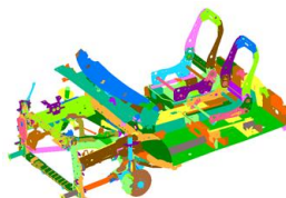
Figure 13: Substructuring for transfer path analysis on a PID level.
